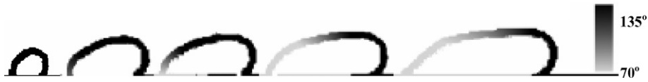
Fig. 17. Predicted side wall contact angle variation during slug growth flow condition: air: 15.56 m/s, water: 0.09 m/s, side wall 135°/70°, bottom: 105°/70°.
